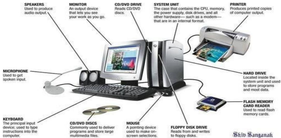
Fig 9.3.1: Components of a computer
