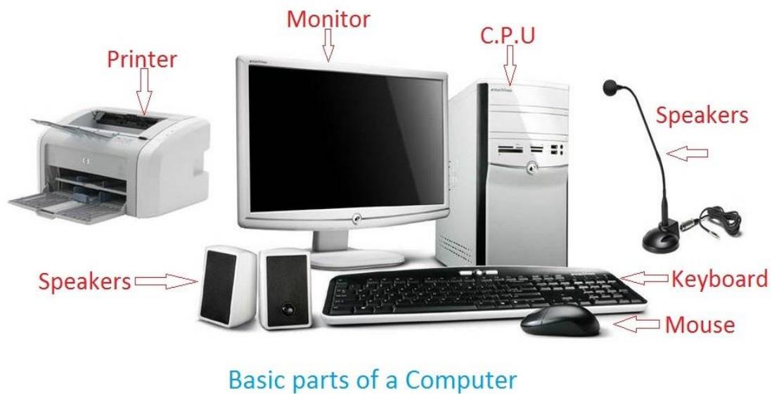
*Fig 9.1.1: Basic parts of a computer*
