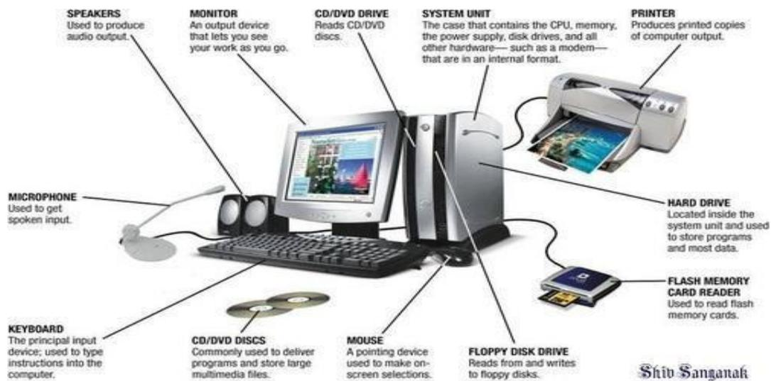
Fig 9.3.1: Components of a computer
